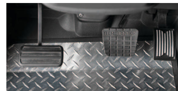
COMFORTABLE PEDALS: The pedals on the Mack® Granite are suspended above the cab floor with the accelerator and brake pedals mounted in-line to reduce operator effort while driving. The clutch pedal is available with air assist, lowering the pedal and greatly reducing driver effort. When combined with our new deep cab and strategically placed seat and steering column, drivers conserve energy and work more productively.
